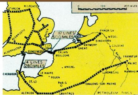
The main network of the PLUTO pipelines. The 500 miles from Dungeness and Greatstone comprised 11 HAIS cables and 6 HAMEL steel pipes
